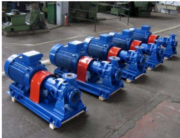
The pumps are horizontal single stage centrifugal pumps - type S10CP25, with the following characteristics: Q=65-111 m3/h, H=82-74 m, and motor P=55 kW n=2900 rpm.
