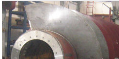
MZT Pumpi's Archimedean screw pump for Skopje wastewater treatment plant
